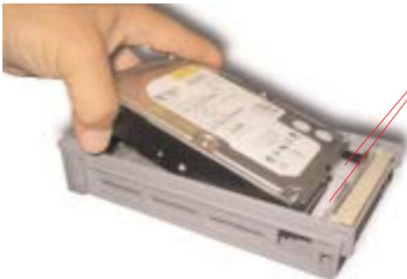
**Plug in the 4 pin power cable and the 40 pin data cable. Both cables have locating tabs so you can not plug them in upside down. Make sure they are completely plugged into their respective sockets. Sometimes rocking the 4 pin cable into its socket makes it easier to insert it.**
