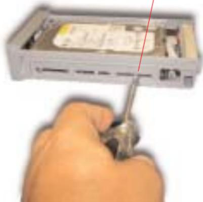
Using a Phillips head screw driver install the (4) mounting screws that hold the drive in place. These screws secure the drive and guarantee that it will be properly grounded when inserted into the system. Do not over tighten the screws. Once the (4) screws are inserted check to make sure that no cables are pinched and that the drive is centered properly.
