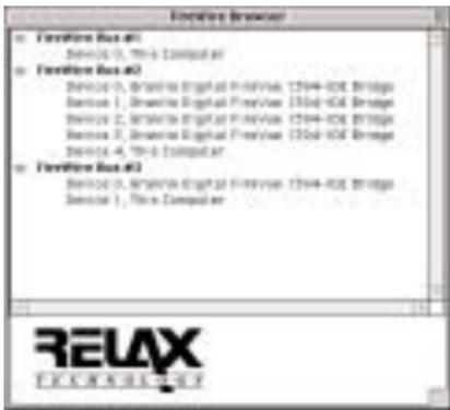
window displays all the available FireWire buses and all the devices that are plugged into that bus. This is the perfect tool to quickly find out if the devices you have plugged in are showing up on the FireWire Bus. Additionally if you double click on the any item in the list, the Browser will give you a long list of information about the device and the manufacturer.
