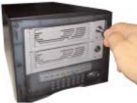
The tray slides back into the Hot-Swap System with very little effort. As the tray reaches the last 1/4 inch, push it in using the handle. The tray will now be flush with the front and has seated properly. Never force the tray into place and always make sure there is nothing in the opening before you insert it.
