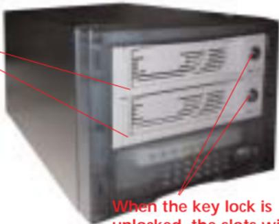
**When the key lock is unlocked, the slots will be lined up at the bottom.**
