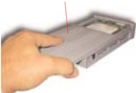
Now reinstall the top of the tray. The side with the notch goes to the front. When sliding the top into place, it will snap into its final position. You are now ready to install the tray back into the Hot-Swap System.
