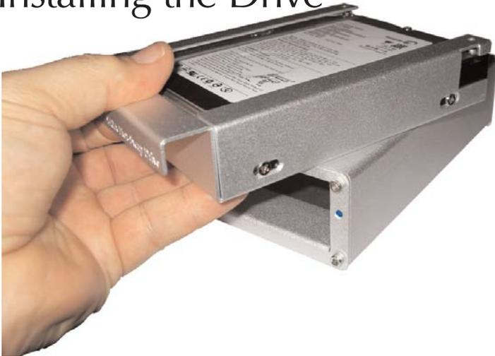
The tray slides back into the Hot-Swap System with very little effort. As the tray reaches the last 1/4 inch, push it in using the handle. The tray will now be flush with the front and has been seated properly. Never force the tray into place and always make sure there is nothing in the opening before inserting it.
