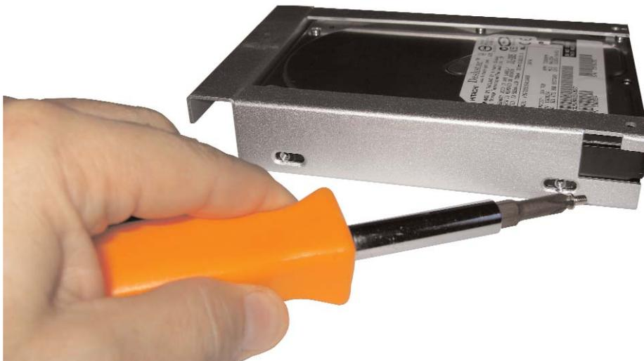
Using a phillips head screw driver install the 4 mounting screws that hold the drive in place. Use only the flat headed phillips screws that are supplied. Make sure they are tight and that the rear of the drive is flush with the rear of the tray.
