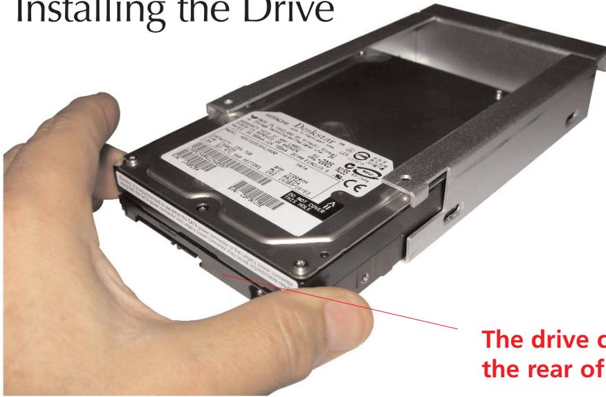
Gently slide the SATA Drive Mechanism in from the rear of the tray. Locate the 4 screw holes and line up the drive mechanism. The drive should be flush with the rear of the tray.
