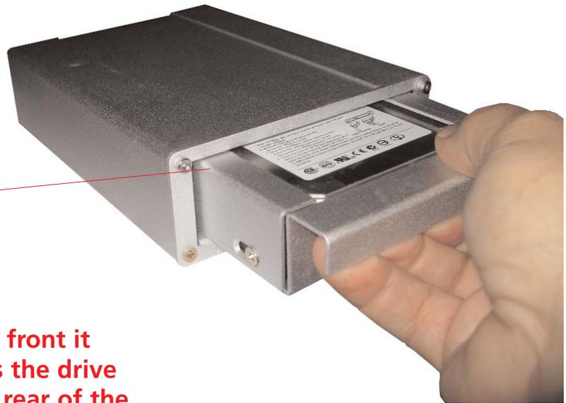
**When the tray is flush with the front it has been inserted correctly. As the drive slides into the connector in the rear of the case you will be able to feel it lock into place.**
