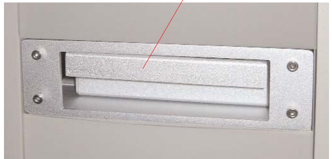
Hot-Swap Drive Trays are easily removed while the computer is on and running. This is truly Hot-Swapable technology.
