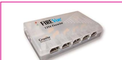
This FireWire 400 1394A HUB / Repeaters allows connections of up to 6 devices. The perfect solution for longer cable needs...simply plug in one of our units and double your cable length. They can also be wired together to offer unlimited capabilities. Power Supply guarantees proper operation of many devices at the same time and rejuvenates the lines.
